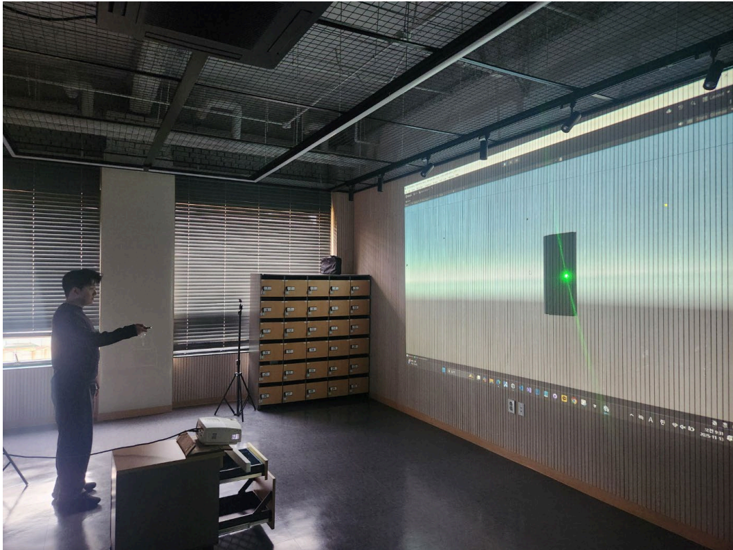
Figure 4. Experimental environment. A participant aims a 532 nm green laser pointer at the projection screen while the Azure Kinect camera (on tripod, left) captures both IR and RGB data. The beam projector is visible in the foreground.
